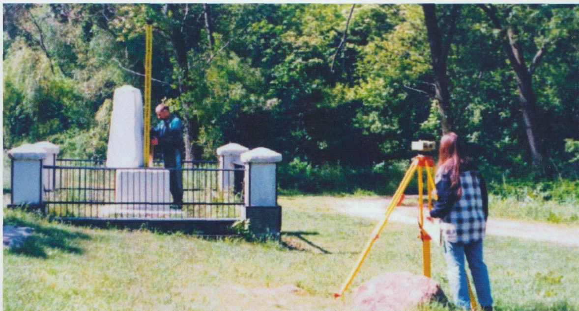
Levelling from Nadap Levelling Nodal Point
